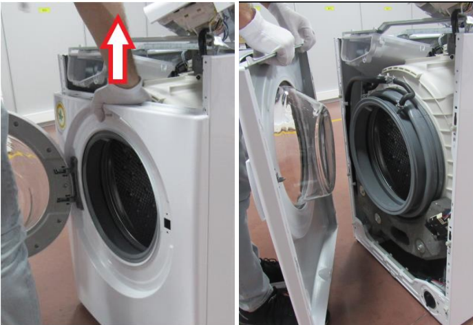
Pull up and remove the front panel.
