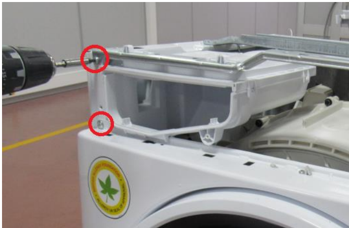
Remove the screw on support bracket and two screws fixing front panel to body
