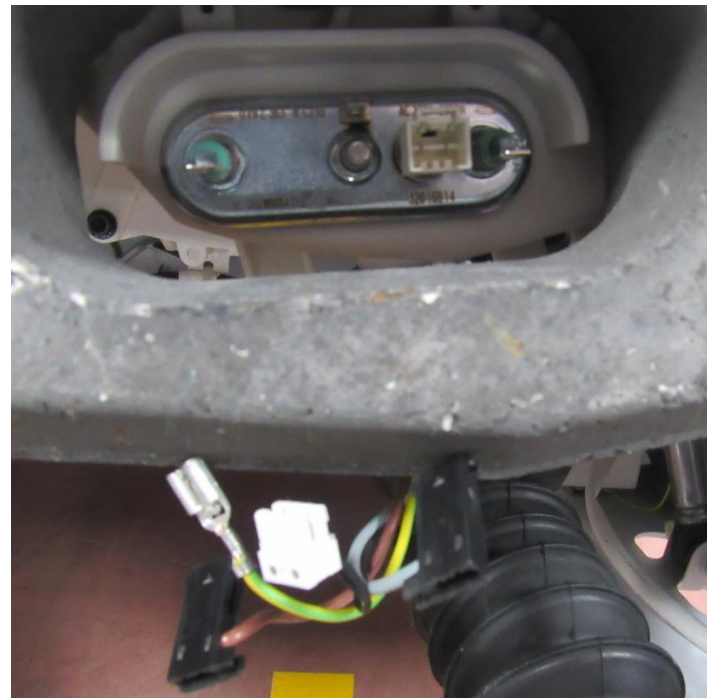
Remove the heater sockets
