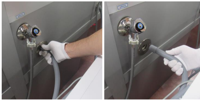
Disconnect the drain hose
