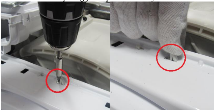
Remove the screw fixing twinjet elbow.
