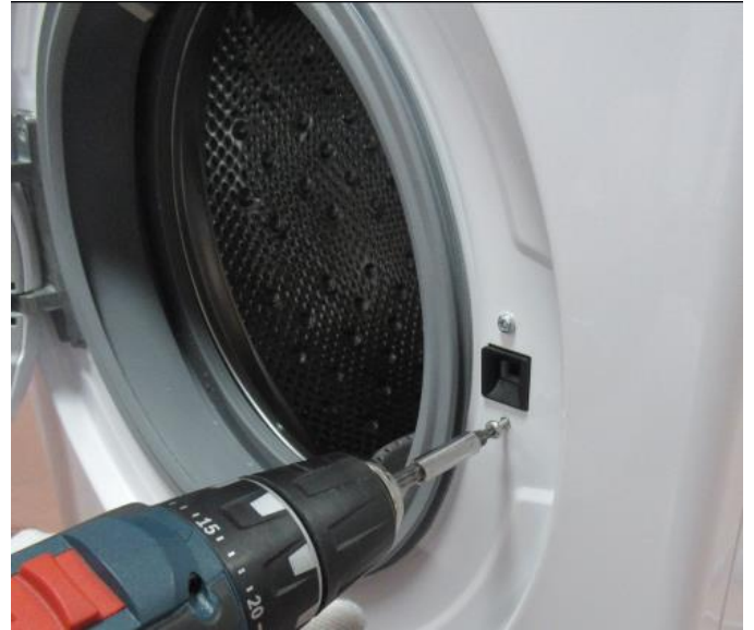
Remove the screws fixing the door lock.
