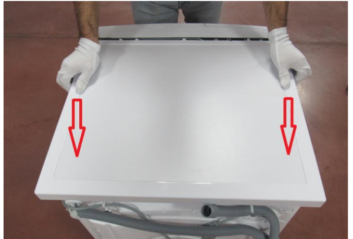
Push the top-plate back and pull it up.
