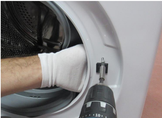
Tighten the door lock screw
