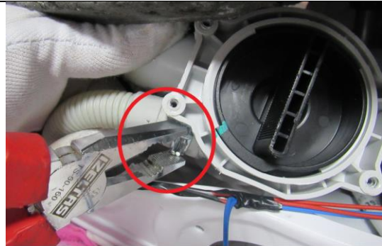
2.15. Remove clamp holding twinjet hose by using a plier.
