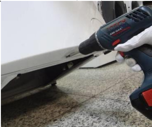
2.8. Remove the screw fixing the front panel at the bottom.
