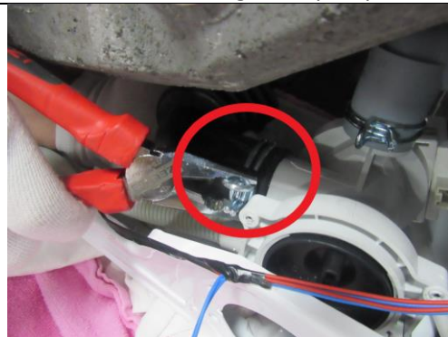
2.13. Remove clamp fixing tub outlet hose by using a plier
