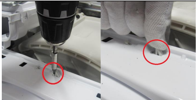
2.5. Remove the screw fixing twinjet elbow.
