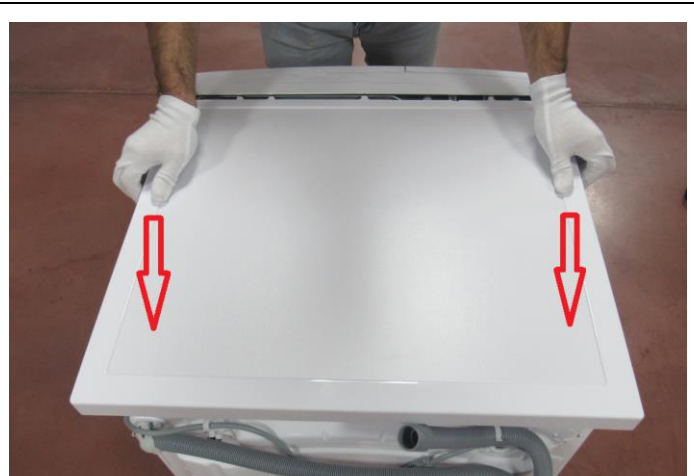
2.2. Push the top-plate back and pull it up.
