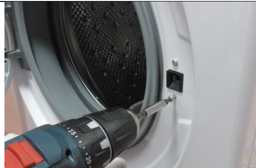
2.6. Remove the screws fixing the door lock.
