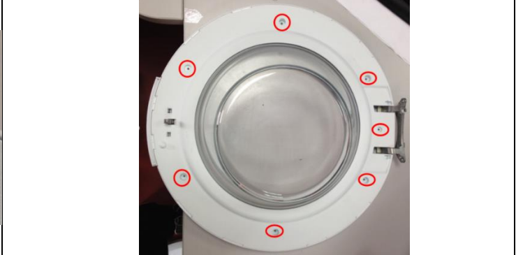
3.13 Assemble the all screws on the inside plastic part of the door.
